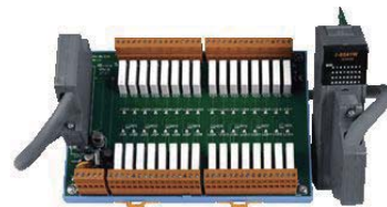
I-87041W, I-87041PW with DN-8K32R and DB37 Male to Female Cable (Optional)
